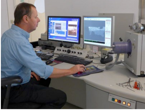
Alan Phenix analyzing a paint sample by SEM-EDS at the Getty Institute
