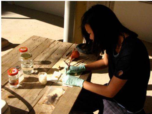
Cybele Tom cleans corrosion from iron in an attempt to better understand the fragment’s original morphology
